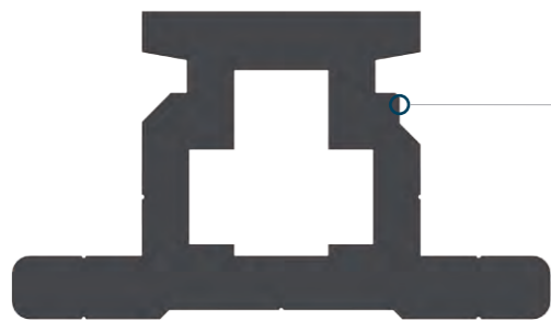
Cross section of rail guide.
